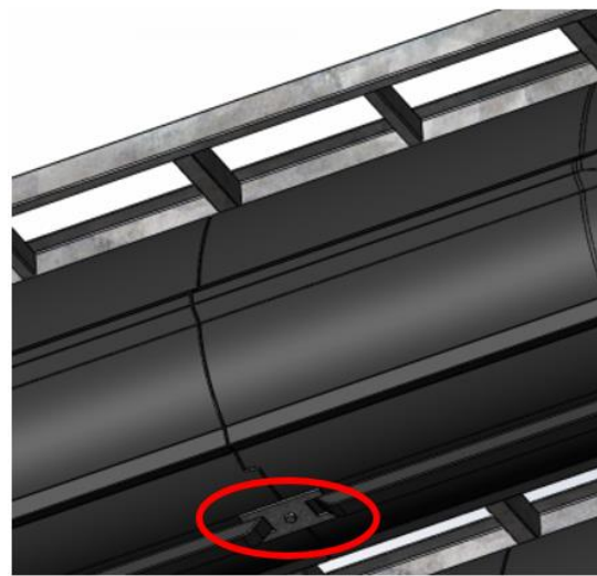
Platform connection with W 1200 S/ W900
